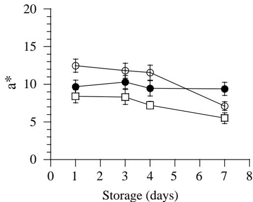
Fig. 5. Evolution of  $a^*$  values for control and pressurized *Biceps femoris* beef samples during a storage at 4°C. Control samples (●), samples pressurized at 130 MPa, 260 s (○) and 520 MPa, 260 s (□), 10°C. The error bars represent the 95% confidence intervals.
