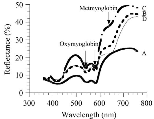
Fig. 4. Reflectance spectra of raw (A), cooked (B), pressurized (C, 520 MPa,  $10^{\circ}\text{C}$ , 260 s) and pressurized then cooked (D, 1 h at  $65^{\circ}\text{C}$ , 520 MPa,  $10^{\circ}\text{C}$ , 260 s) *Biceps femoris* beef samples.
