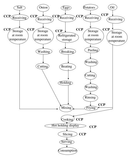
Fig. 1. Flow diagram of Spanish potato omelette in restaurants (CCP: critical control point).
