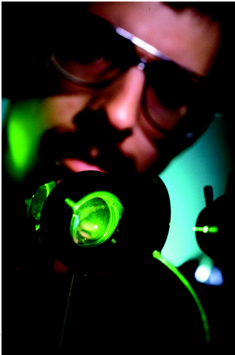
Optical biosensor developed by the U.S. Dept. of Agriculture allows the measurement of aflatoxin or fumonisin in corn.
