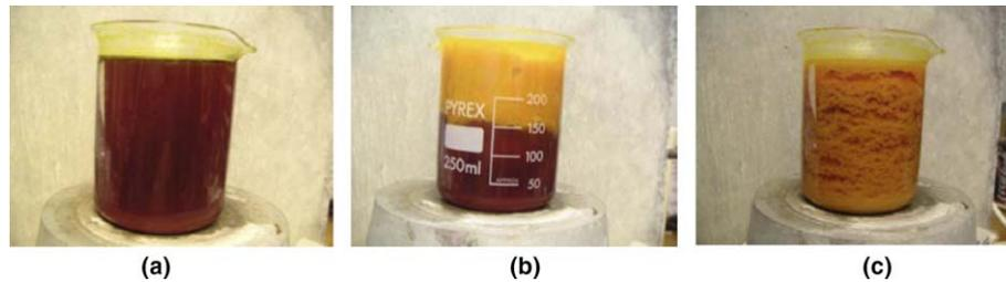
Fig. 4. Photograph of palm oil at different times during the experiment of Fig. 3, taken at (a) 0 min (60 °C), (b) 115 min and (c) 175 min (22 °C).
