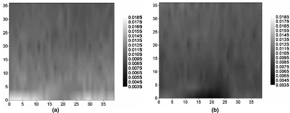
Fig. 10. Non-contact through-transmission imaging of banana milk with pH 5 in a Plexiglas container. (a) Image of sample immediately after it has been injected with acid and (b) image obtained 1 h later, indicating regions of coagulation throughout the sample.
