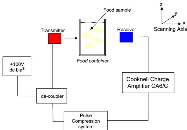
Fig. 1. Apparatus for measuring changes in liquid foods within a Plexiglas container using non-contact air-coupled ultrasound.
