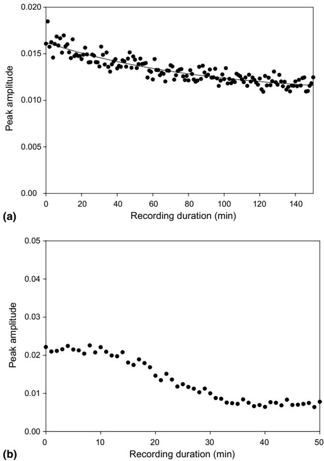
Fig. 7. Variations of peak through-transmitted ultrasonic amplitude with time after treatment with acid at pH 5 for (a) full-fat milk and (b) strawberry-flavour milk drink.
