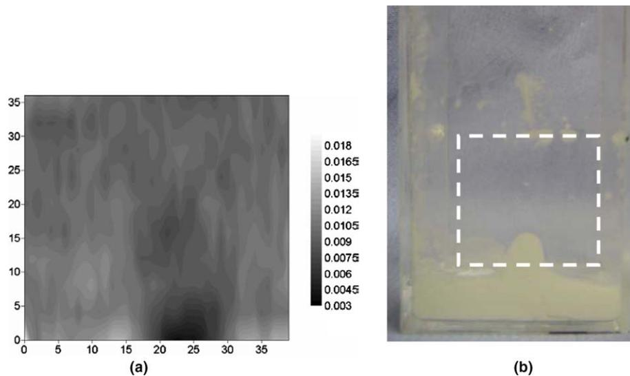
Fig. 8. Non-contact through-transmission imaging of the full-fat milk sample mixed with sulphuric acid. (a) Cross-sectional image formed by scanning the air-coupled ultrasonic system and (b) a photograph of the Plexiglas container showing the resultant coagulated milk attached to the base.
