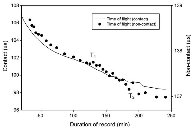
Fig. 5. Variation of ultrasonic time-of-flight across palm oil as temperature changes from  $T_1$  of 33 °C to  $T_2$  of 22 °C.  $T_1$  and  $T_2$  denote phase transitions.
