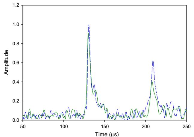
Fig. 6. Comparison of received ultrasonic signals after processing with pulse compression, following propagation across a Plexiglas container filled with either 3.6% full-fat milk (dashed line) or strawberry milk (solid line).
