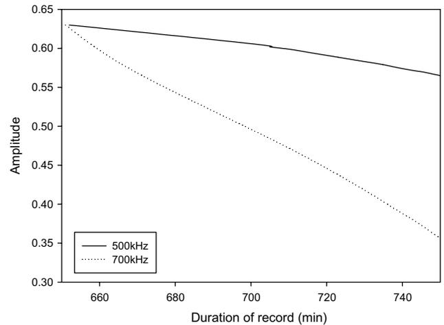
Fig. 2. Change in air-coupled through-transmitted ultrasonic signal amplitude at centre frequencies of 500 kHz and 700 kHz with time, for a palm oil sample. This was cooled and crystallised from a temperature of 60 °C.
