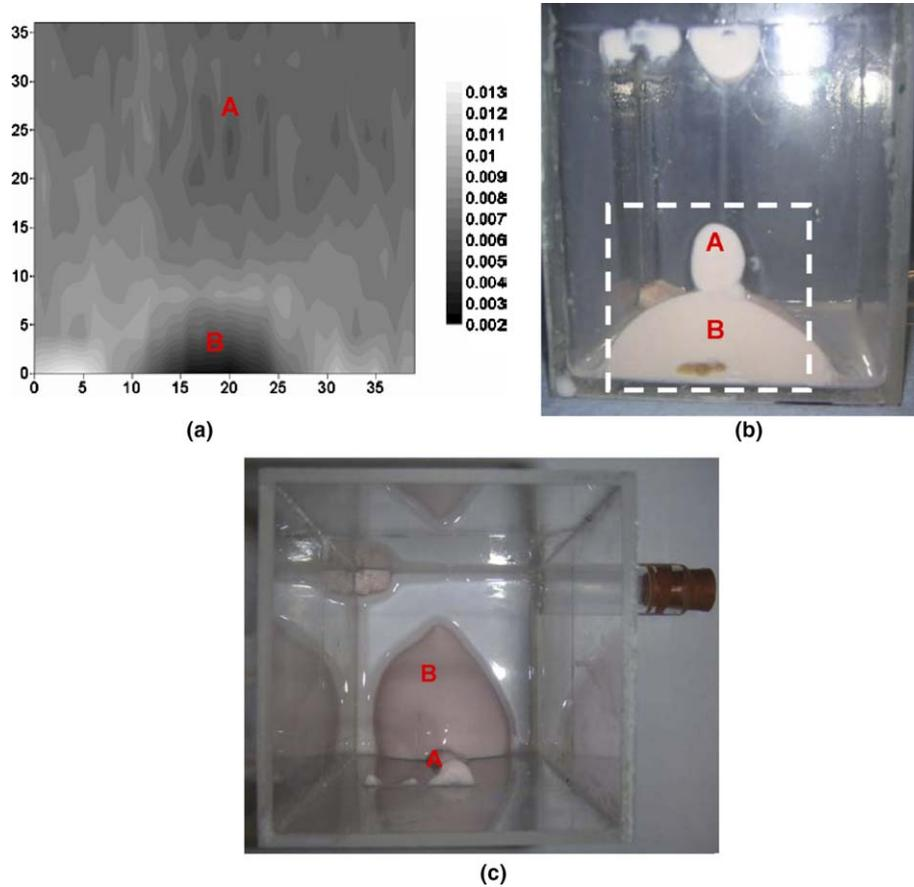
Fig. 9. Non-contact through-transmission imaging of the strawberry-flavoured milk drink, after being mixed with sulphuric acid and left for 20 min. (a) Cross-sectional scan using the air-coupled ultrasonic system, (b) photograph (side view) showing the coagulated region attached to the base of the container and (c) top view of the emptied container.
