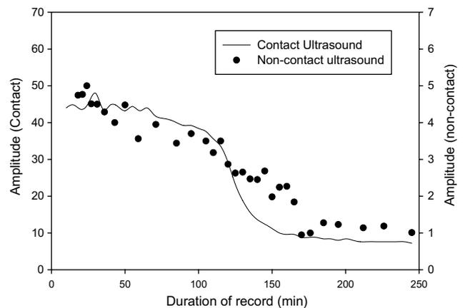
Fig. 3. Comparison of signal amplitudes produced by both contact measurements (continuous line) and non-contact air-coupled measurements (dots) as a function of time, as palm oil was cooled from 60 °C to room temperature.
