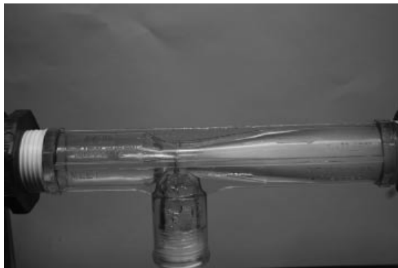
Figure 4.7 Venturi injector in operation. (Courtesy of Mazzei Injector Corp., Bakersfield, CA.)
