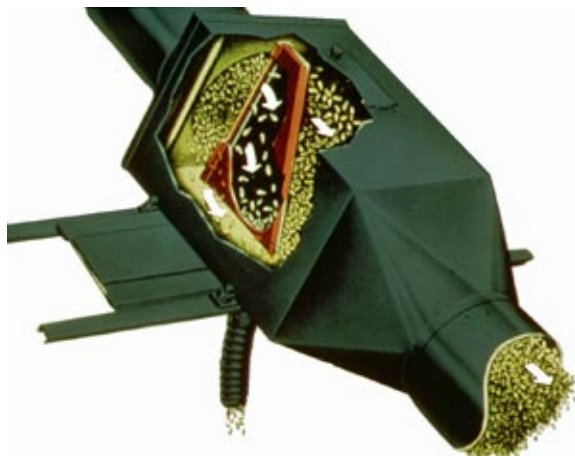
Figure 2. Diverter-Type sampler installed in spout.
