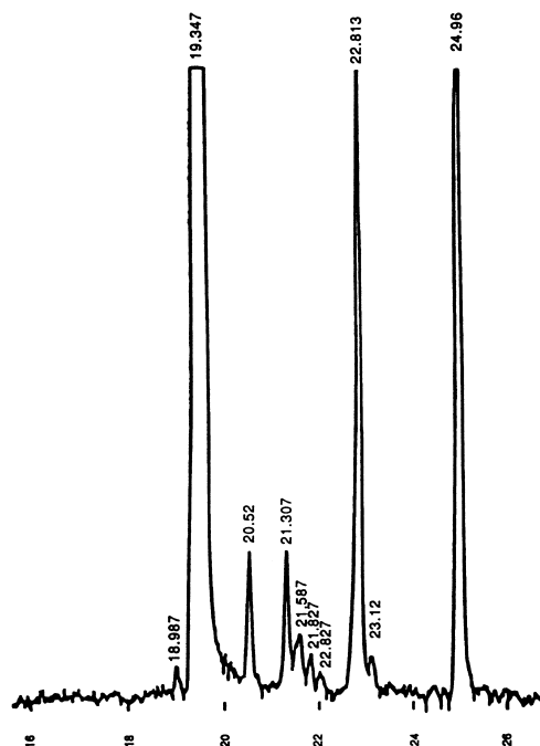
Fig. 5. Truncated Varex LC–ELSD chromatogram from a 4- \mu l injection of a ‘dirty’ FB 1 sample dissolved in water at 3.03 \mu g/ \mu l. (Reprinted by permission from Ref. [98].)
